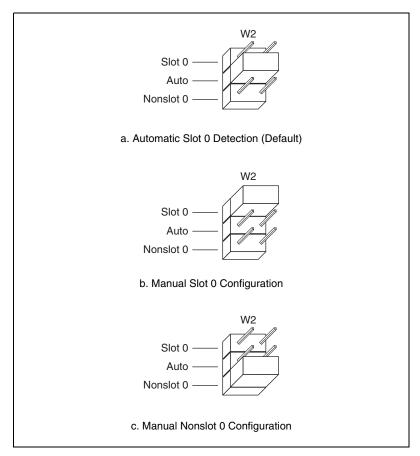
Figure 3-3. VXIbus Slot Configuration
